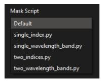
The included mask scripts allow you to filter on a single wavelength or reflection index, or simultaneously filter for two.
